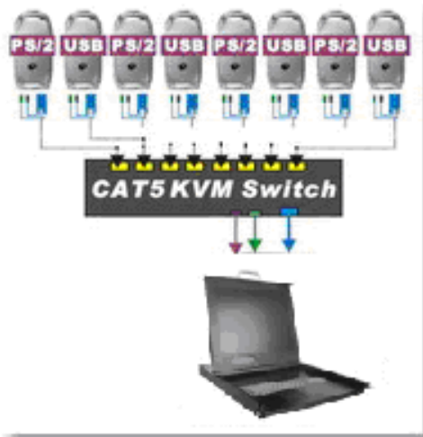
8-Port Rack-PS/2&USB double interface CAT5 KVM computer switch connection diagram
